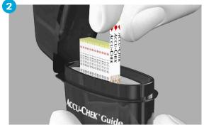
**SIDE PINCH.** Grasp the sides of the outermost test strip with a pinching action as you pull up.
