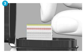
**PINCH AND PULL.** Place your index finger on top of the test strips. Then with your thumb, press in against the test strips and slide the front test strip up to pull it out in one motion.
