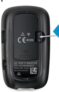
To insert new batteries, open the child-resistant battery door by inserting a narrow object into the slot, pushing the tab in the direction of the arrow, and lifting the door up.
