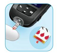
Wait for the screen to show apply blood and then touch the **yellow edge** of the test strip to the blood drop.
