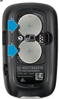
Slide the new batteries under the black tabs and button, with the **(+) side facing up**. Put the battery door back in place and snap it closed.
