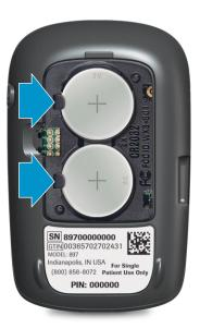
Slide the new batteries under the black tabs with the (+) side facing up.
