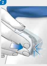
Fit the recess on the micropump onto the hook on the pump holder.
