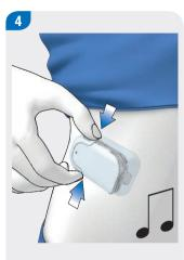
If the acoustic feedback corresponds to the desired insulin amount and you want to deliver the quick bolus, press both quick bolus buttons simultaneously until you hear the sequence of signals for delivering the bolus.
