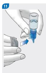
Remove the filling aid from the reservoir by pulling it off laterally in the direction of the arrow.
