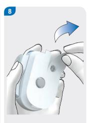
Remove both parts of the protective film from the adhesive pad.
