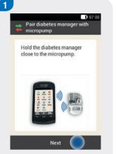
After you have connected the reservoir to the pump base, hold the diabetes manager close to the micropump to establish the radio connection.
