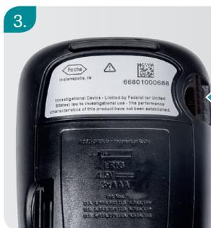
With the code number facing away from you, reinsert the code chip into the Meter until it stops.
