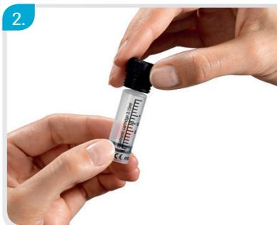
Push the adapter (thread-part first) all the way onto the cartridge tip to the stop.
