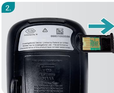
Turn the Meter display-side down. Remove the code chip, turn it over and check the code written on the chip is 222.
