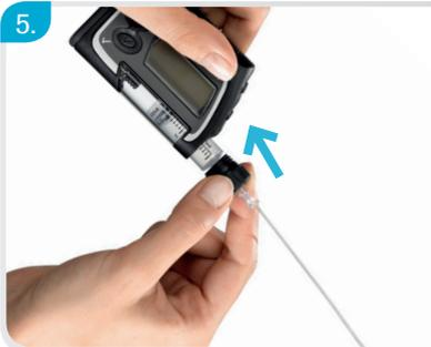
5. Hold your Pump diagonally with the adapter pointing down. Insert the cartridge into the cartridge compartment.
