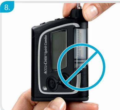
8. If the end plate of the piston rod is not correctly aligned with the cartridge plunger, remove the cartridge from the cartridge compartment and repeat steps 1. to 6.
