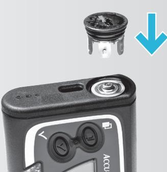
Place the cover on the positive end and gently push the battery in, while turning the cover clockwise to partially tighten it.
