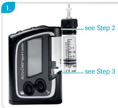
Hold the Pump upright. Hold the new filled cartridge so that the connected adapter and infusion set point upwards, parallel, and close to the cartridge compartment.
