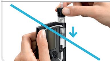
Do NOT hold your Pump upright when inserting the cartridge. This could lead to insulin flowing into the cartridge compartment and cause a blockage of the piston rod. The Pump may then display an E6 or E10 error message or stop.
