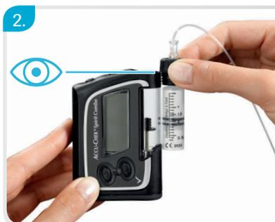
Make sure that the top edge of the threaded part of the adapter is level with the top part of the cartridge compartment.
