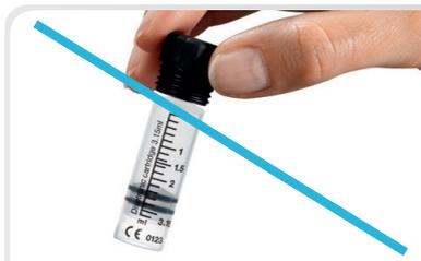
Do NOT insert the cartridge into the insulin pump without the infusion set tubing connected. This could lead to insulin flowing into the cartridge compartment. If insulin gets into the compartment this can result in a damage of the piston rod over time and potentially limit or cause a blockage of the insulin pump motor functions.
