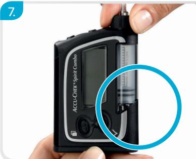
7. The cartridge is correctly inserted when the end plate of the piston rod is correctly seated against the cartridge plunger.
