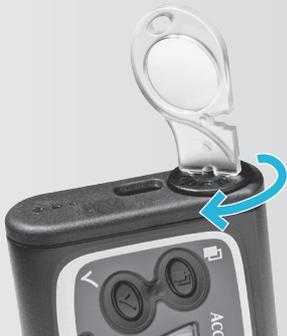
Use the battery key to fully tighten the battery cover.
