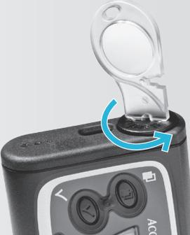
Remove the battery cover, using the battery key to turn the battery cover anti-clockwise.
