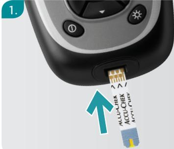
1. Place your Meter on a flat surface (for example, a table) and insert the test strip into the Test Strip Slot in the direction of the arrow. The Meter turns on.
