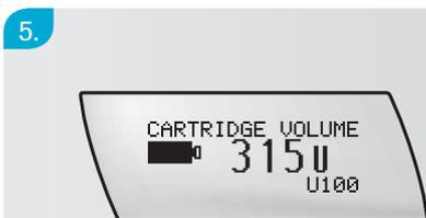
When the piston rod has returned completely, the CARTRIDGE VOLUME screen displays the maximum volume, 315 U.
