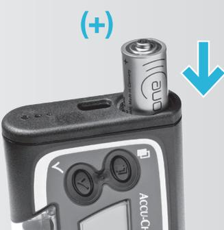
Insert the battery, negative (-) end down, positive (+) end up, into the compartment.
