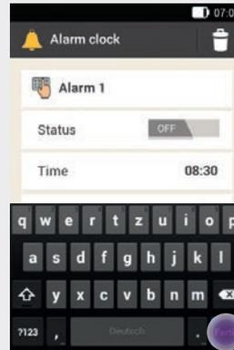
Enter a name for the alarm clock reminder using the keyboard. The name may have up to 15 characters.
