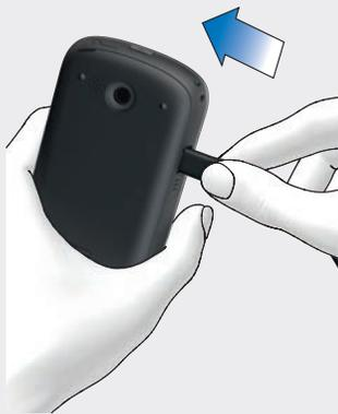
Plug the smaller end (micro-B plug) of the USB cable into the USB socket of the diabetes manager.
