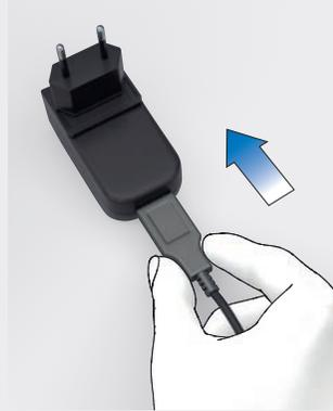
Plug the larger end (USB type A) of the USB cable into the USB socket of the charger.
