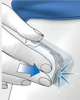
Using pressure on the pump shield, press the micropump onto the pump holder until there is a clearly audible **CLICK**.
