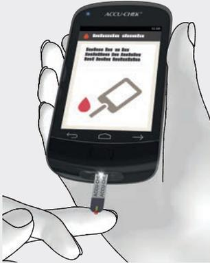
Touch the blood drop to the front yellow edge of the test strip.
