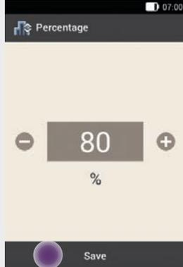
Use **-** and **+** to set the percentage for adjusting the Temporary Basal Rate.
