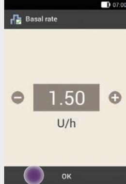
The screenshot shows the 'Basal rate' screen with a basal rate of 1.50 U/h. There are minus and plus buttons on either side of the rate display, and an 'OK' button at the bottom.
