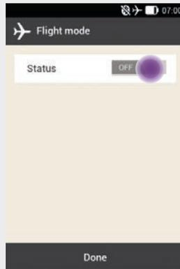
Tap **Status** to put the switch in the **OFF** position.
