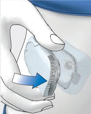
Fit the recess on the micropump onto the hook on the pump holder.
