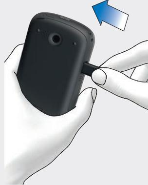
Plug the smaller end (USB type micro-B) of the USB cable into the USB socket of the diabetes manager.
