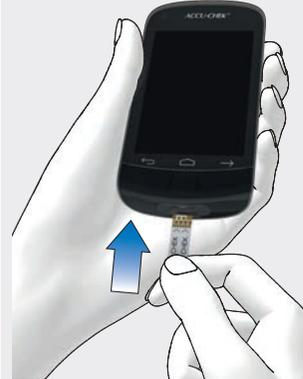
Insert the test strip into the test strip slot of the diabetes manager in the direction of the arrow. The device turns on automatically and the LED at the test strip slot lights up. If the tone for blood glucose tests is turned on, a signal sounds.
