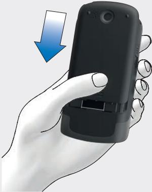
Close the battery compartment by pushing the battery door in the direction of the arrow until it clicks into place.
