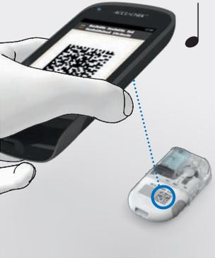
Point the camera of the diabetes manager at the pairing code on the pump base. Hold the diabetes manager in such a way that the pairing code can be read in full. A signal sounds if the pairing code was detected, and a prompt to fill the reservoir needle is displayed.
