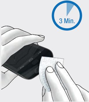
Wipe the surface of the diabetes manager for at least 3 minutes using a second, lint-free cloth moistened with demineralised water. Clean in particular hard-to-reach places, for example, around the openings.
