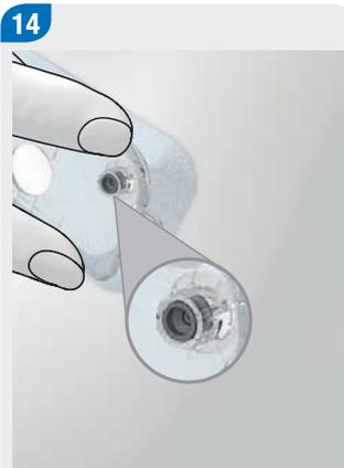
Check whether the grey cannula head in the cannula opening is visible and flush with the opening.
