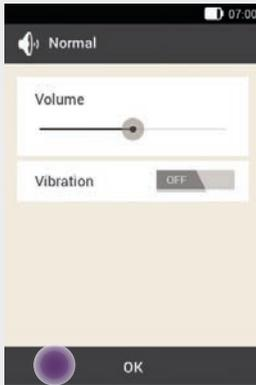
Set the volume for the default setting by moving the slider.
