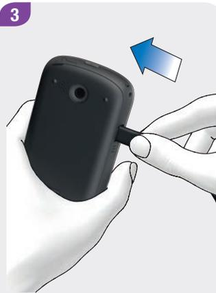
Plug the smaller end (micro-B plug) of the USB cable into the USB socket of the diabetes manager.
