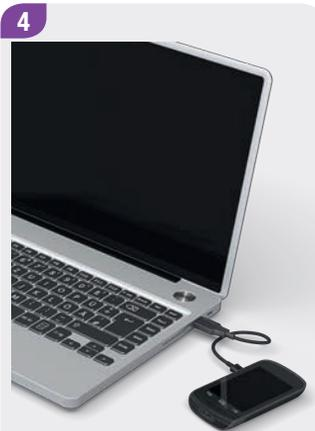
Plug the larger end (USB-A plug) of the USB cable into a free USB port on your computer.
