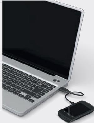
Plug the larger end (USB-A plug) of the USB cable into a free USB charging port on your computer. The USB charging port is often indicated by a lightning bolt symbol ⚡.
