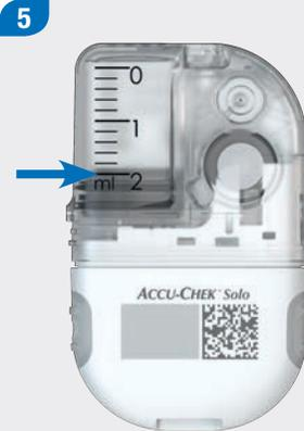
Read the reservoir level using the reservoir scale.
