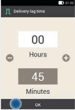
Use **-** and **+** to set the delivery lag time. The delivery lag time can be 0, 15, 30, 45 or 60 minutes.
