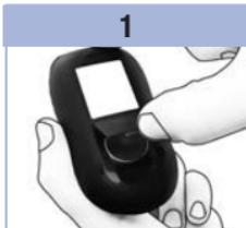
Open the battery door on the back of the meter by pushing the tab in the direction of the arrow and pulling the door up.
